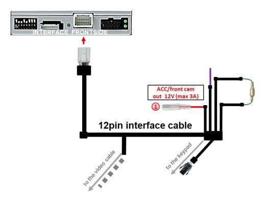
1 The red power supply output ACC/front cam out 12V (max 3A) can be used to power an external source and has a different assignment depending on the position of dip switch 1 (of the black 8 dips):
