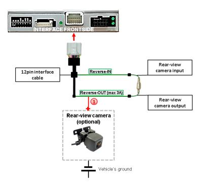
1 The 12 V power supply for the rear-view camera (max 3A) has to be taken from the green wire of the 12pin interface cable to avoid an unnecessary, permanent power supply to the camera electronic.
