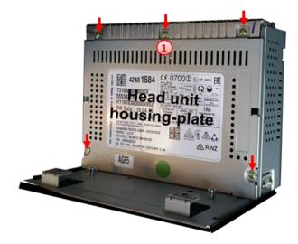
Remove the head-unit and further remove the original housing cover plate, which is fixed to the head-unit housing by 5 Torx screws (T9).
