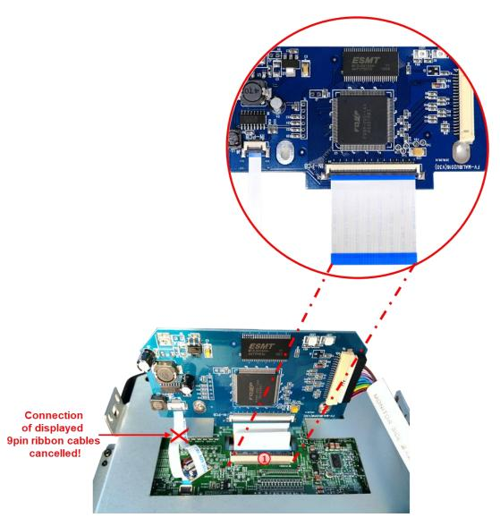
Connect the daughter PCB's pre-assembeled 66pin ribbon cable "IN PCB" to the previously become free ribbon cable base of the monitor mainboard (heed the following warning notes!).
