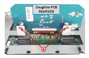
After connecting the ribbon cables, the daughter PCB has to be fixed with its rearside at the exchange retaining plate by using the enclosed 2 shorter screws.
