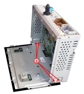
Turn out the 4 screws of the monitor retaining plate.
